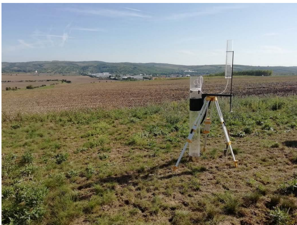
Fig. 5: Measurement of infiltration properties on the anti-erosion grass strip
