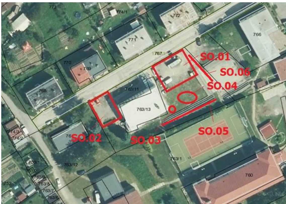
Fig. 1: Location of individual proposed objects of green infrastructure in the village of Drienov (SO.01 Main green semi-vegetated area, SO.02 Side green semi-vegetated area, SO.03 Underground retention tank, SO.04 Raingarden, SO.05 Vegetation retaining wall, SO.06 Belt of greenery)
